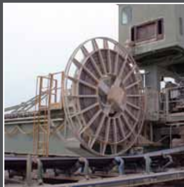
Level Wind Reel on a Stacker/Reclaimer, USA
