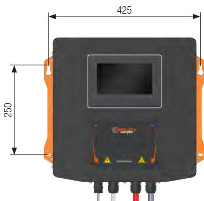
Drilling pattern for wall mounting
